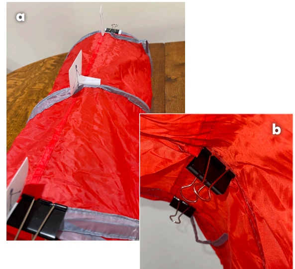
FIGURE 6. BINDER PLACEMENT FOR GPS IMAGES. (a) Attach the two end GPS stations using binder clips from the open tunnel ends. (b) Attach the middle GPS image using a binder clip from the inside.
