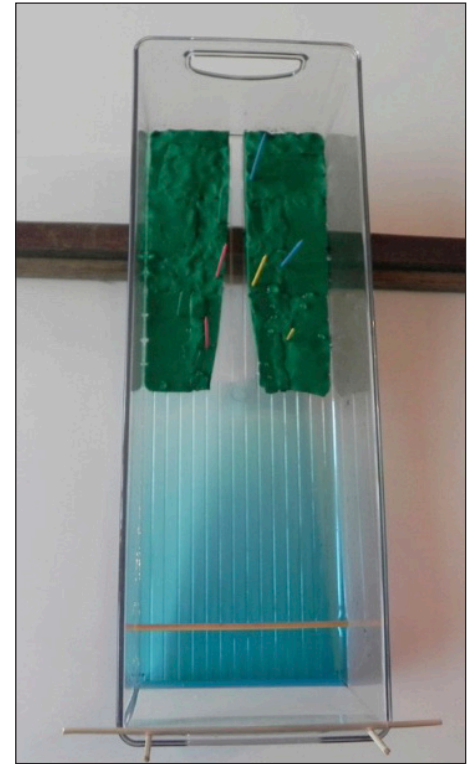
Figure B: View looking into the wave container. The variable in this example is a narrow inlet perpendicular to the coastline that is wider at the mouth. In this example, toothpicks mark points on the landscape.
