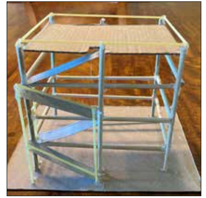
Figure 2: Example of a Tsunami Vertical Evacuation Structure (TVES) tower model.
