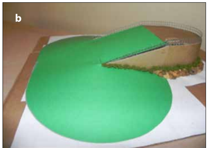
Figure 5: a) Classroom model of tsunami vertical evacuation tower showing stairways and b) berm designs with a broad ramp designed to deflect floating debris.
