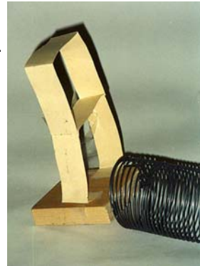
Fig. 3. Photograph of slinky attached to a small wood block and cardboard "house." The slinky could also be attached to the bottom of the wood block to illustrate P- and S-waves propagating upwards and shaking the building. The slinky is attached to the wood block using screws and washers using the same method illustrated in Figures 4-6.
